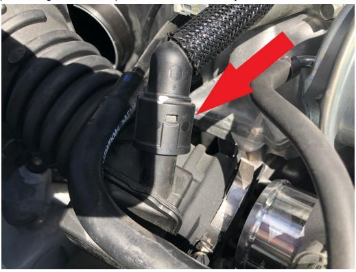
3. Using a flathead screwdriver, remove the clamps on the air intake tube.
