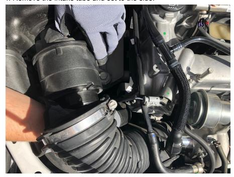
5. Locate the bypass valve. It is located just below the turbocharger inlet, where you just removed the intake hose. Disconnect the electrical connector on the bypass valve by using a small flat head screwdriver to lift up on the connector lock, then pull the connector off.
