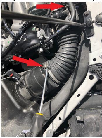
4. Remove the intake tube and set to the side.
