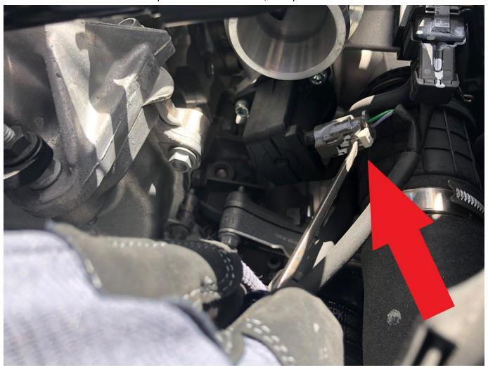
6. Remove the 3 machine screws/bolts holding the bypass valve to the turbo. They are H5 hex keys but a 3/16 allen key will also work. We've already removed them in the image, but you can see where they were. The 3rd screw is not visible, but the arrow is there to represent where it is on the other side of the valve.
